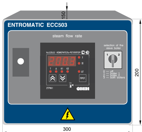
Fig. 21. Overall dimensions, mounting holes of ECC503
